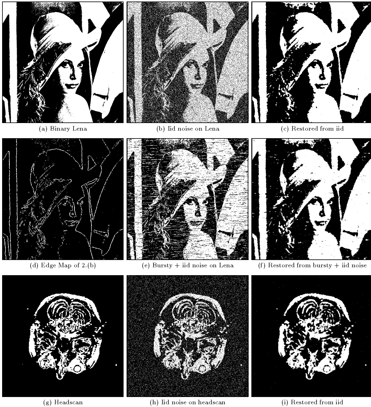
Figure 2: Restoration of images with a combination of iid and bursty noise using contagion urn schemes.
