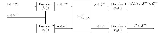
Figure 1: Transmitting two CS over the asymmetric 2-user communication channel.
