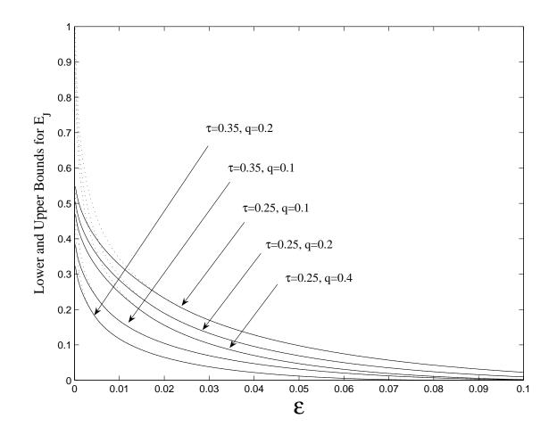
Figure 2: The lower bound (solid line) and the upper bound (dash line) for the system JSCC error exponent for transmitting binary CS over the binary AMAC with binary additive noise.
