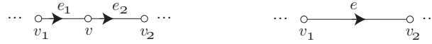
Fig. 4.8 If we remove the vertex v from a graph we replace the edges e_1 and e_2 by the edge e . (See Definition 17.)
