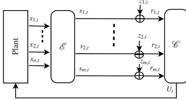
Fig. 1.2 Control over a point-point channel
