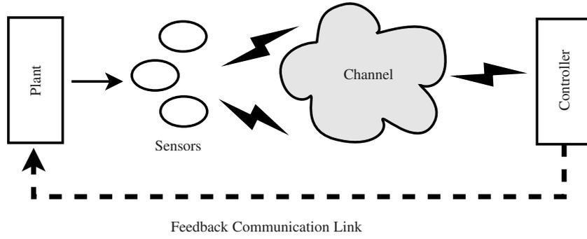
**Fig. 1.1** Feedback control over sensor network
