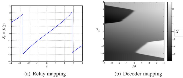
**Fig. 1.19** Relay and decoder mappings ( $K_1 = K_2 = 1$ ) optimized for  $\sigma_x^2 = P_s = P_r = 1$  and  $\gamma_{ed} = 5$  dB,  $\gamma_{er} = 10$  dB, and  $\gamma_{rd} = 25$  dB.
