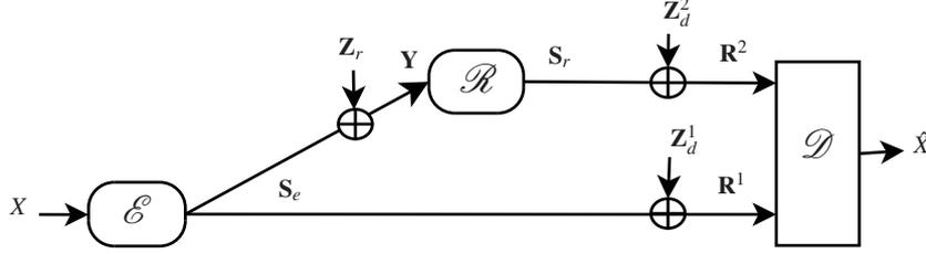
**Fig. 1.18** Real-time transmission of a Gaussian source over an orthogonal half-duplex Gaussian relay channel.
