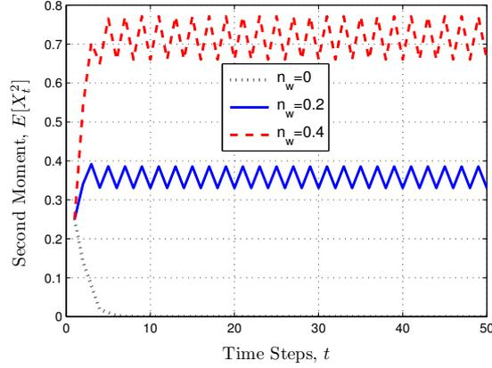
**Fig. 1.8** Comparison of second moments of the plant state process at three different levels of process noise.
