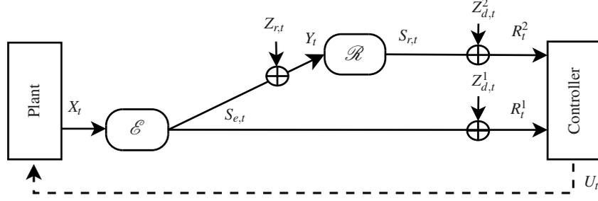
**Fig. 1.11** Orthogonal half-duplex AWGN relay channel.
