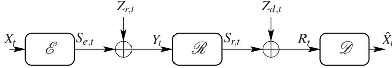
**Fig. 1.15** Real-time transmission of a memoryless Gaussian source over a two-hop relay channel.
