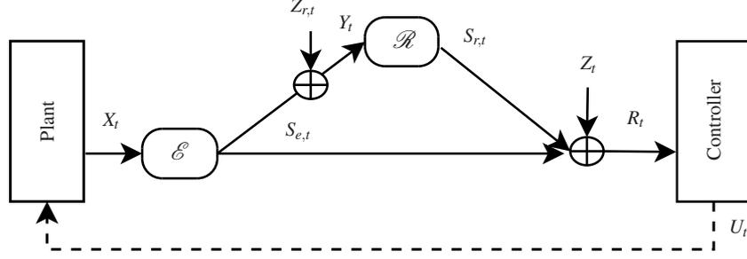
Fig. 1.10 Non-orthogonal full-duplex AWGN relay channel.
