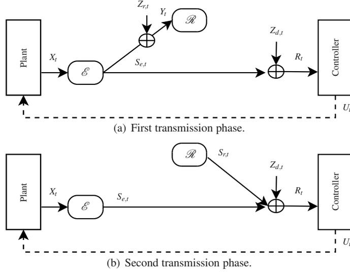
**Fig. 1.7** Half-duplex AWGN relay channel.
