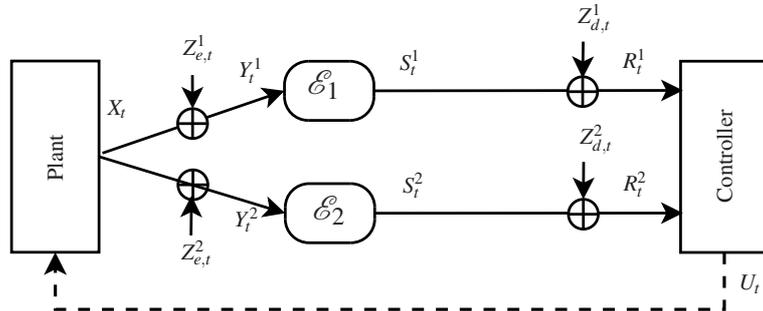
**Fig. 1.24** A closed-loop control system with state measurements transmitted over wireless channels.
