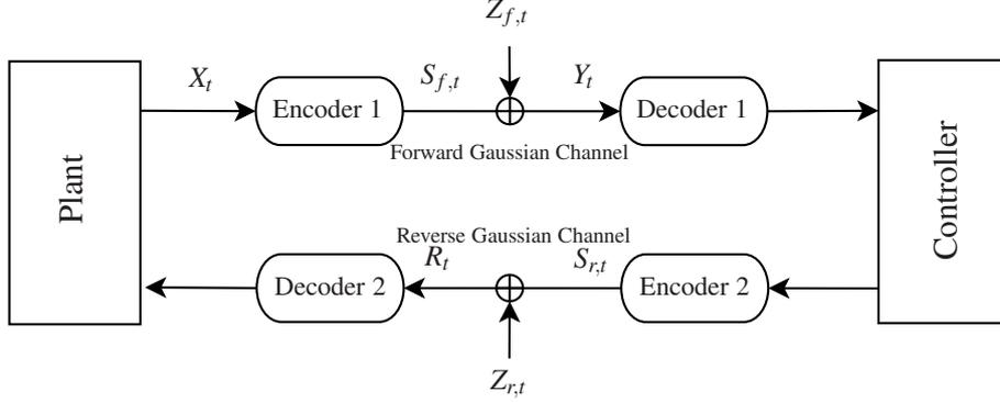
**Fig. 1.3** Stabilization over noisy forward and reverse Gaussian channels.
