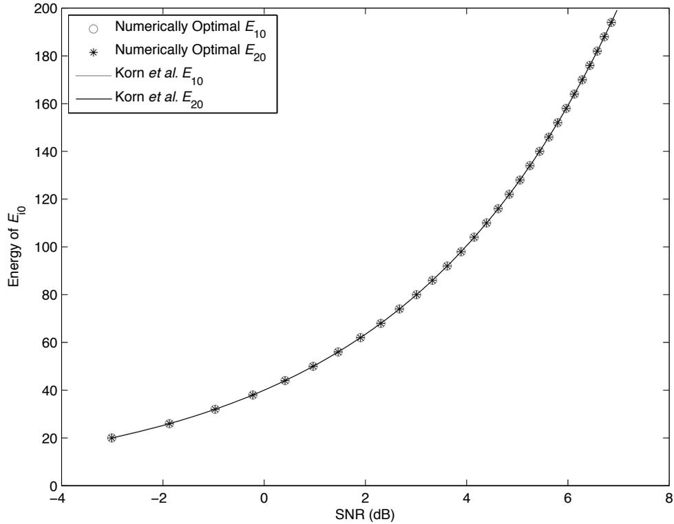
Figure 4.7: Numerical optimization vs. results in [1] when  $\gamma = 1$  and  $E_{10} = E_{20}$ .
