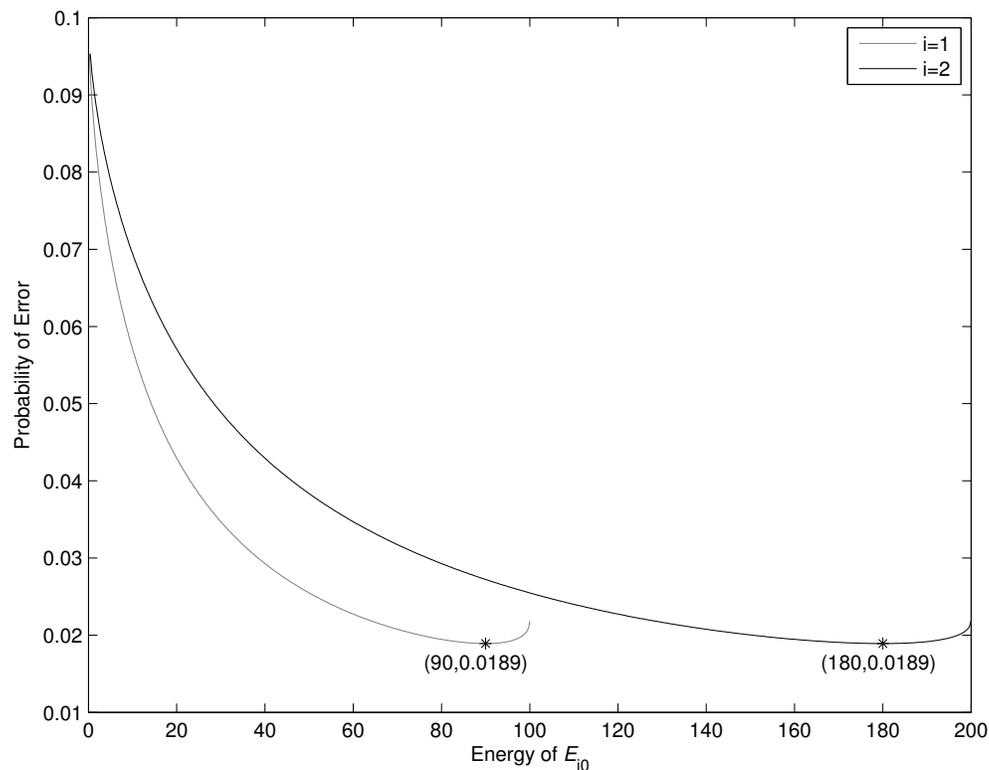
Figure 4.6: Numerical optimization when  $\gamma = -1$  and  $2E_1 = E_2$ .
