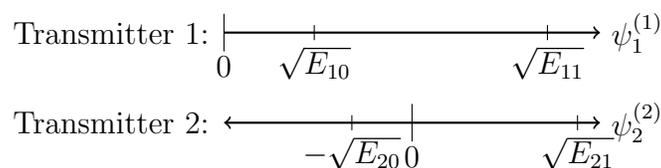
Figure 3.4: Modulation scheme for Transmitter 1 and 2 when  $\gamma_1 = -\gamma_2 = 1$ .
