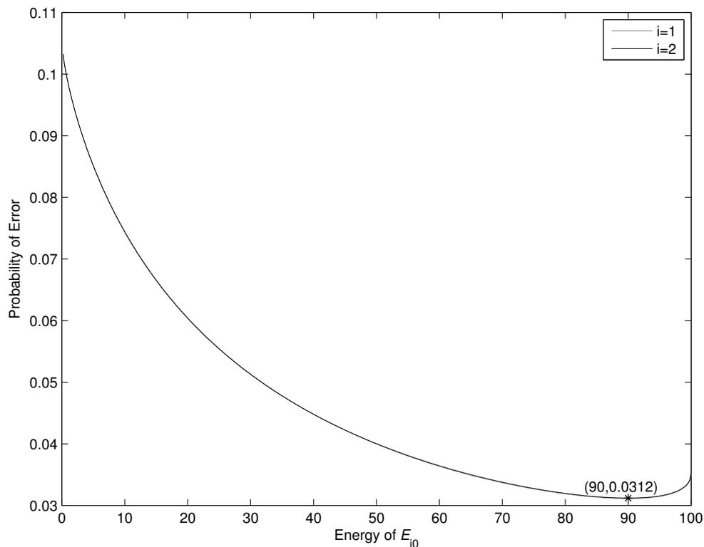
Figure 4.5: Numerical optimization when  $\gamma = -1$  and  $E_1 = E_2$ .
