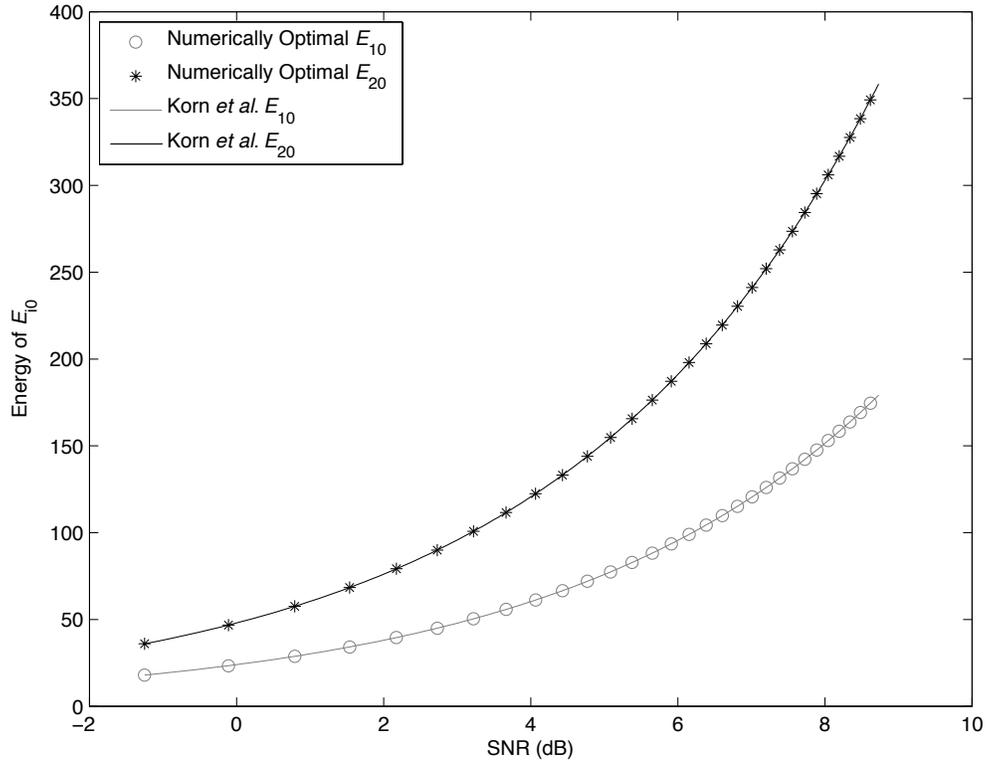
Figure 4.10: Numerical optimization vs. results in [1] when  $\gamma = -1$  and  $2E_{10} = E_{20}$ .
