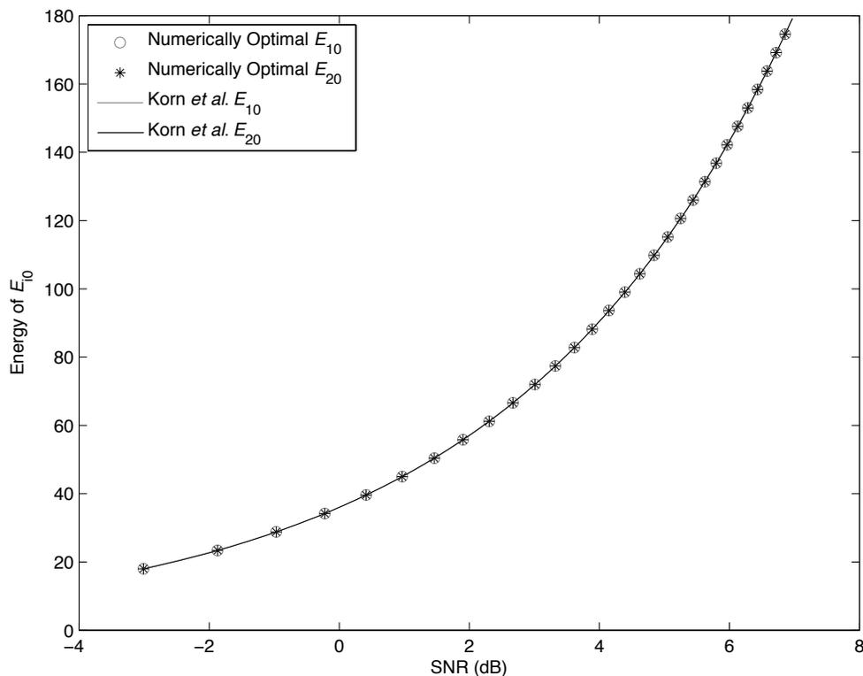
Figure 4.9: Numerical optimization vs. results in [1] when  $\gamma = -1$  and  $E_{10} = E_{20}$ .
