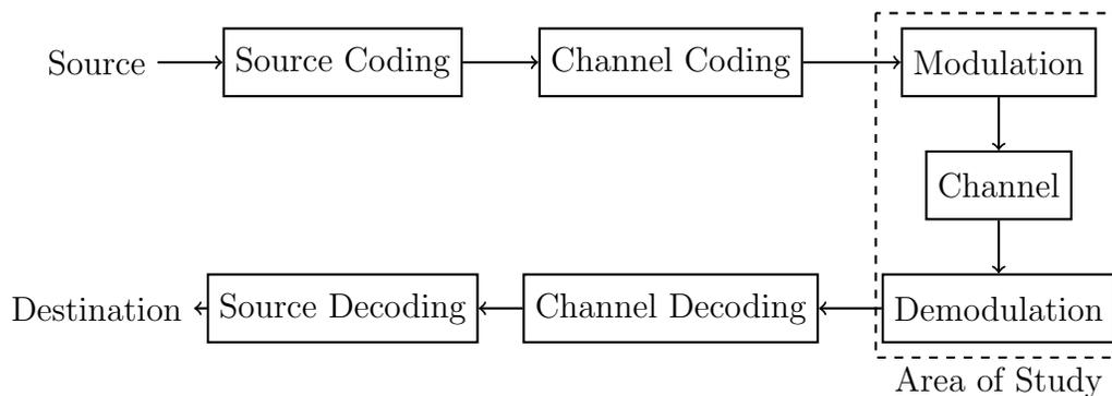
Figure 1.1: Block diagram representing the components of a communication system, with a highlighted area of the topic relevant to this document.
