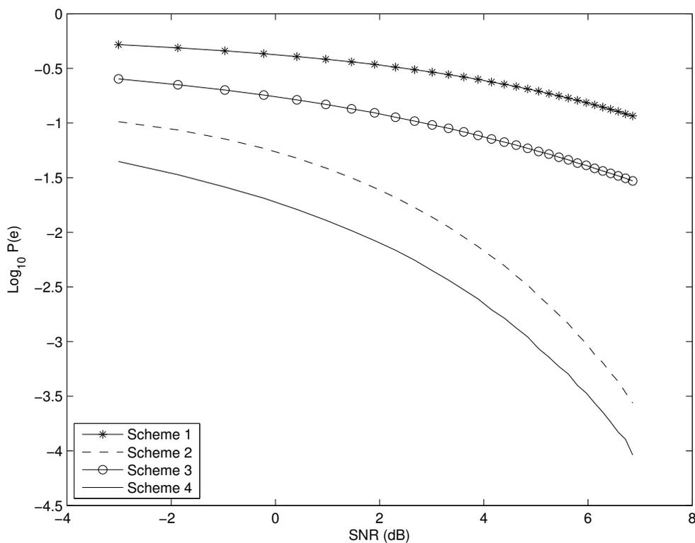
Figure 4.11: Comparison of schemes when  $\gamma = 1$  and  $E_1 = E_2$ .
