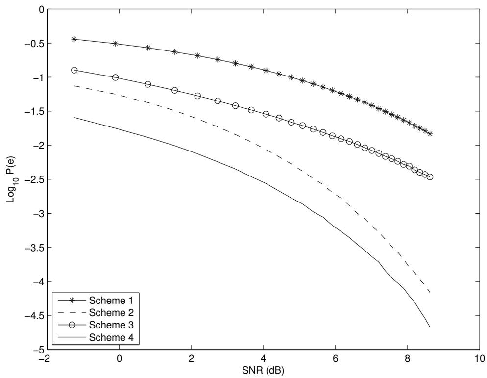
Figure 4.15: Comparison of schemes when  $\gamma = -1$  and  $2E_1 = E_2$ .
