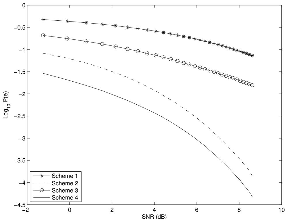
Figure 4.12: Comparison of schemes when  $\gamma = 1$  and  $2E_1 = E_2$ .
