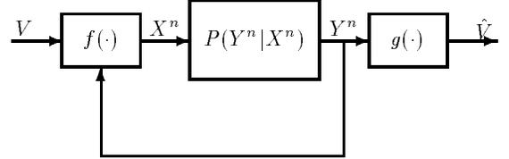
Figure 2. Block diagram of a channel with feedback.
