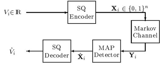
Figure 2. Block Diagram of Joint Source-Channel Coding System Using MAP Detection.
