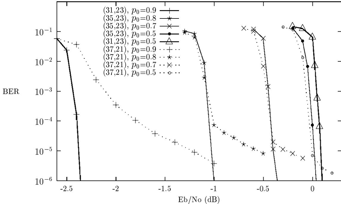
Figure 1: Turbo codes for non-uniform i.i.d. sources,  $R_c=1/3$ ,  $N=262144$ , AWGN channel.
