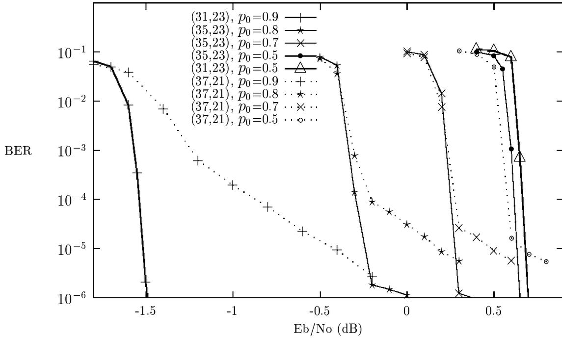
Figure 2: Turbo codes for non-uniform i.i.d. sources,  $R_c=1/2$ ,  $N=262144$ , AWGN channel.
