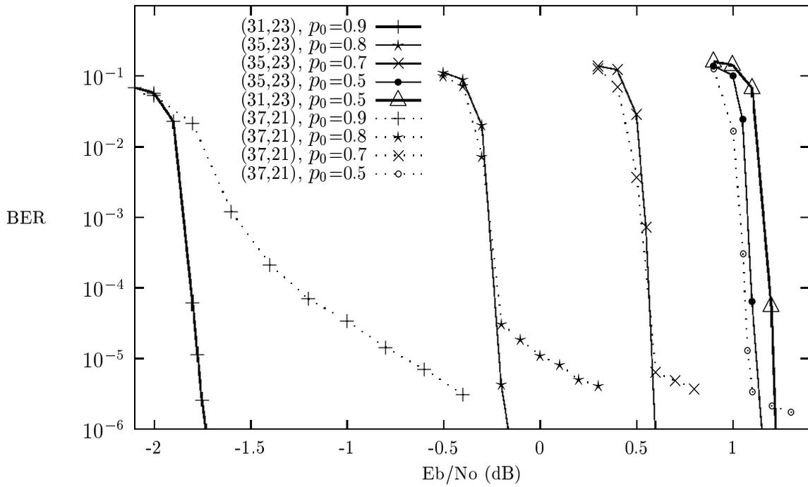
Figure 3: Turbo codes for non-uniform i.i.d. sources,  $R_c=1/3$ ,  $N=262144$ , Rayleigh fading channel.
