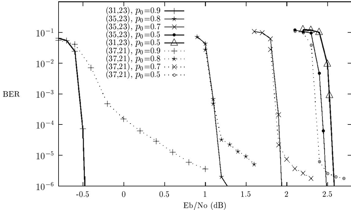
Figure 4: Turbo codes for non-uniform i.i.d. sources,  $R_c=1/2$ ,  $N=262144$ , Rayleigh fading channel.
