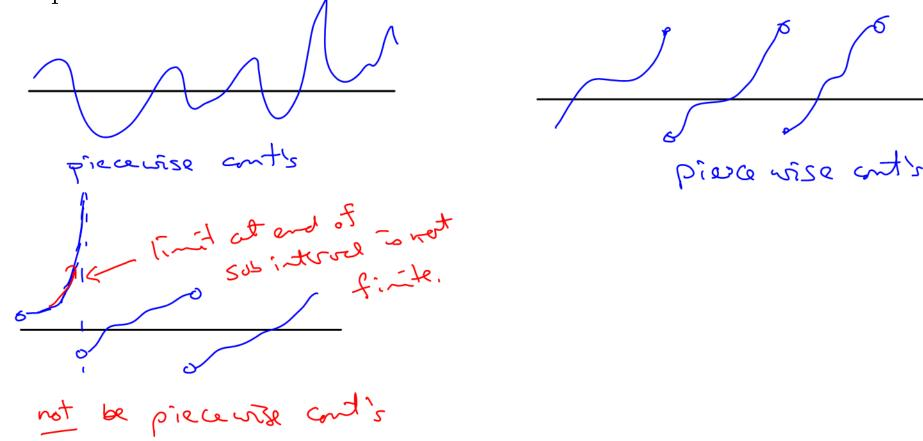
One of the requirements for a function having a Laplace transform is that it be piecewise continuous. Classify the graphs above based on this criteria. Another requirement of the Laplace transform is that the integral  $\int_{0}^{\infty} e^{-st} f(t) dt$  converges for at least some values of  $\underline{s}$ . To help determine this, we introduce a generally useful idea for comparing functions, "Big-O notation".
