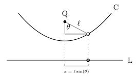
(b) The distance from the object to the line L is the distance from Q to the line, minus the distance that the object is below Q, or  $d - \ell(t) \cos(t)$ . The distance from point Q to the object is  $\ell(t)$  (this is the definition of  $\ell(t)$ !).
