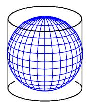
Then projection "sideways" from the vertical axis of the sphere onto the surface of the cylinder is an area preserving projection. I.e., whatever shape you draw on the surface of the sphere, when you project it onto the cylinder it may end up distorted, but it will still have the same area.
