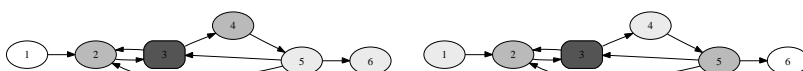
Figure 2.1: The sets \overline{\mathcal{P}}_{3 \rightarrow} (left) and \overline{\mathcal{P}}_{\leftarrow 3} (right) for an example connection graph. Patches directly connected to 3 appear in darker gray, indirectly connected patches appear in lighter gray. Patches with no access to 3 or that cannot be accessed from 3 are white.
